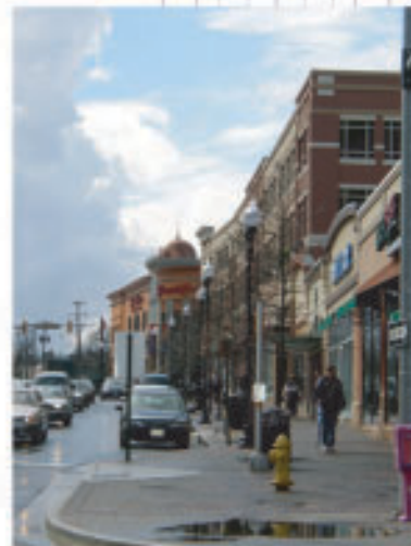
Bulb-out and on-street parking
